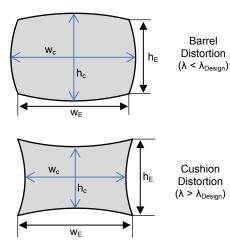
$\theta_H$ = horizontal angle,  $\theta_V$ = vertical angle,  $h_C$ = center height,  $w_C$ = center width,  $h_E$ = edge height,  $w_E$ = edge width
